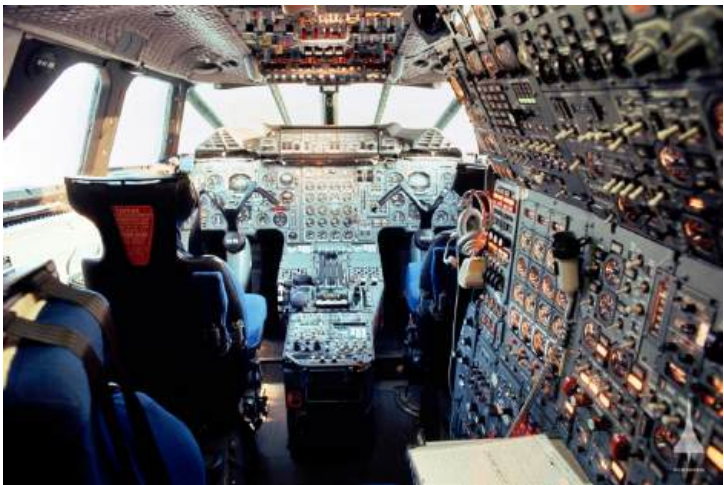
The Concorde’s cockpit was a compact, highly technical environment designed for a three-person crew: two pilots and a flight engineer. Unlike modern glass cockpits, Concorde’s flight deck was filled with hundreds of analogue dials, switches, and gauges, each essential to managing the aircraft’s complex systems—particularly the variable-geometry air intakes and the powerful Olympus 593 engines. Photo: ©Collection Musée Air France.
